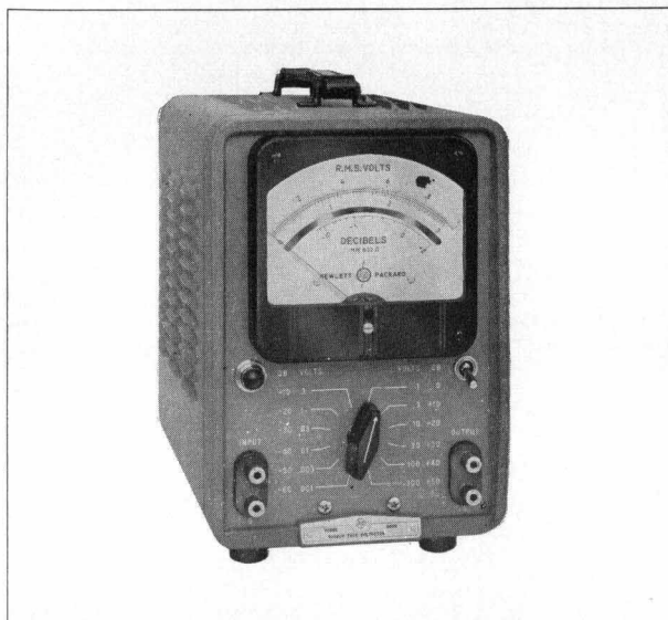
Fig. 1. New -hp- Model 400H VTVM has 1% accuracy over 50 cps-500 kc range, 2% accuracy over 20 cps-1 mc range, is usable to 4 mc. Mirror scale and high-definition meter contribute to accuracy of reading.
